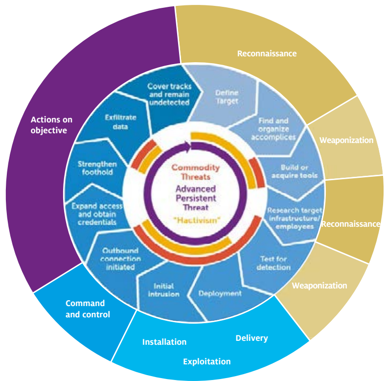
Figure 2: Mapping Dell SecureWorks (inner circle) and Lockheed Martin (outer circle) targeted attack kill chain.
