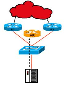
Figure 7: First Hop Redundancy principle
