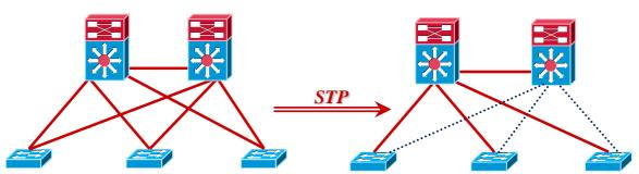
Figure 11: Spanning Tree Protocol effect on switched LAN
