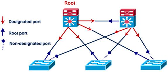
Figure 12: Converged Spanning Tree and port statuses
