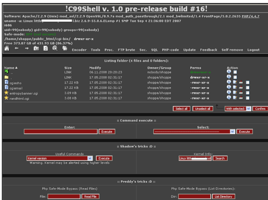
Figure 56: Example of a C99 shell script viewed in the browser (source: https://3.bp.blogspot.com/-VbGMAncOcz4/Vjxck9Npxnl/AAAAAAAAEaw/ThnZkYMhrRc/s1600/get%2Bc99%2Bshells%2Bfrom%2Bgoogle.png )
