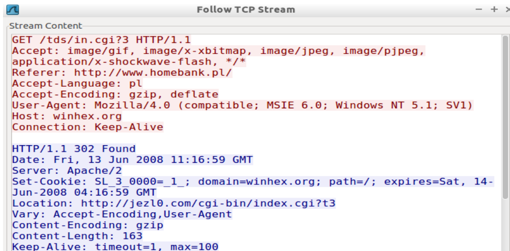
Figure 30: Follow TCP stream in Wireshark.
