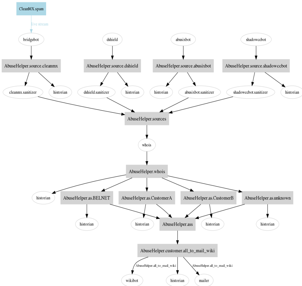
Figure 2: AbuseHelper workflow structure ( https://www.cert.be/files/demolayout3.png ) 6
